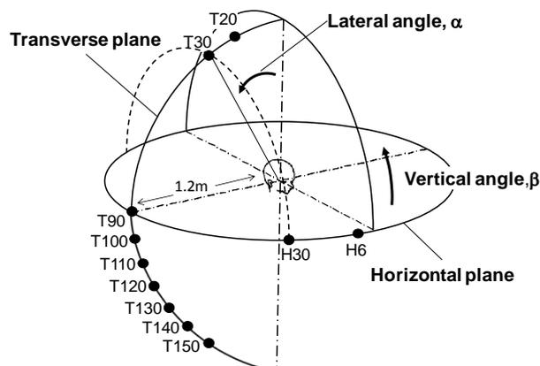
Fig.1 Loudspeakers arrangements in the horizontal plane (H30 and H6) and in the transverse plane (T20 - T150).
