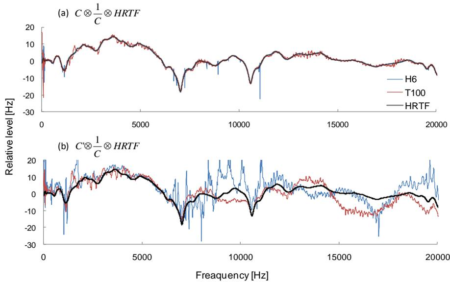
Fig.5 Simulated HRTF by transaural system. (a): transfer function is constant, (b): listening position is changed.
