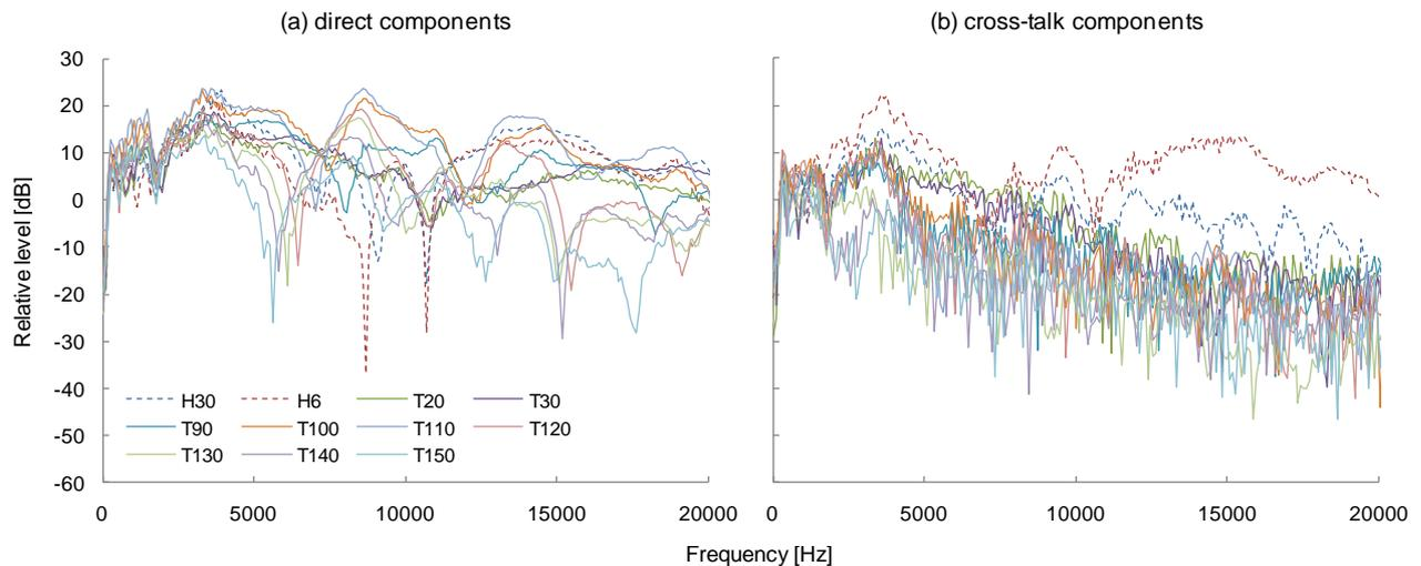
Fig.2 Transfer functions between the loudspeakers and the entrance of the ear canal of a subject. (a) direct components between the left loudspeakers and the left ear, (b) cross-talk components between the left loudspeakers and the right ear.
